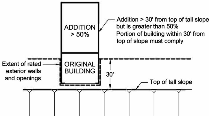
PLAN VIEW SHOWING WHEN BUILDING MUST COMPLY WITH VCBC SECTION 456.3
