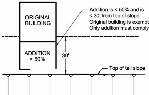
PLAN VIEW SHOWING WHEN ADDITION MUST COMPLY WITH VCBC SECTION 456.3
