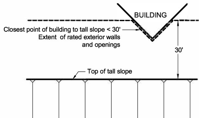
PLAN VIEW SHOWING WHEN BUILDING MUST COMPLY WITH VCBC SECTION 456.3
