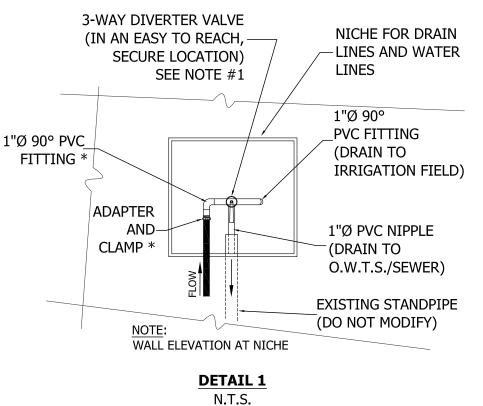
\* IRRIGATION PIPING LEADING TO THE DISPOSAL AREA MUST NOT BE SMALLER THAN THE WASHER HOSE.
