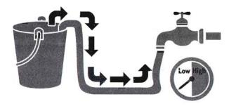
Backsiphonage occurs when pressure drops in the drinking water system.
