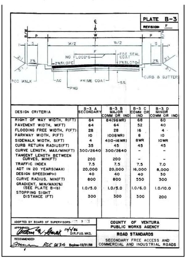
Figure P-16 1986 County Road Standards Plate B-3
