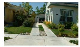
**Driveways with pervious strips** down the center allow for extra infiltration and capture of transportation-related pollutants.
