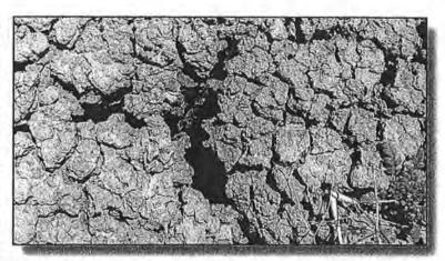
Fig. 2. Close up photo of calcareous heavy clay soil, cracked and shrunk during the dry season.
