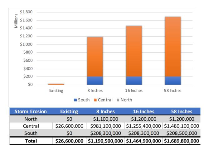
**Figure 5-1. Estimated cumulative value of property loss due to erosion by planning area with a 1% annual chance storm (2017 dollars).** *Note: Only bluff erosion was modeled for the South Coast, and erosion was not modeled for the North Coast due to the existing shoreline armory.*
