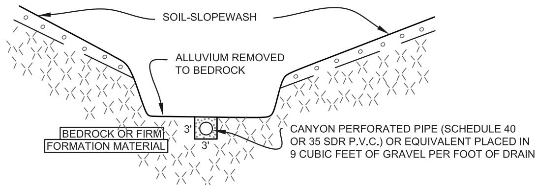
GRAVEL TO CONFORM TO CALTRANS CLASS 2 PERMEABLE MATERIAL AS ALTERNATE 3/4" GRAVEL MAY BE USED SURROUNDED WITH GEOTEXTILE FILTER FABRIC APPROVED BY THE GEOTECHNICAL ENGINEER.
