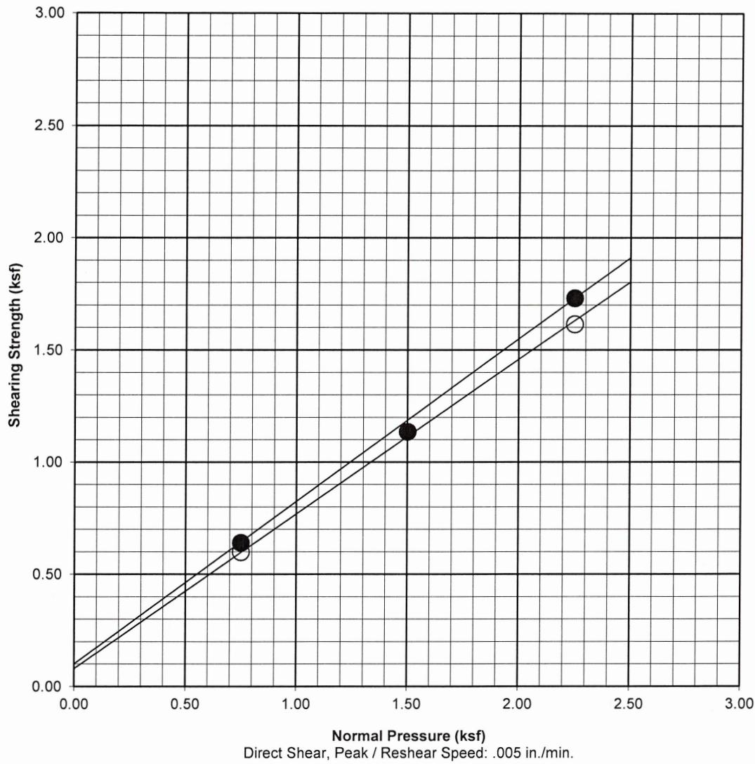
Sample Remolded to 90% Relative Density, saturated.
