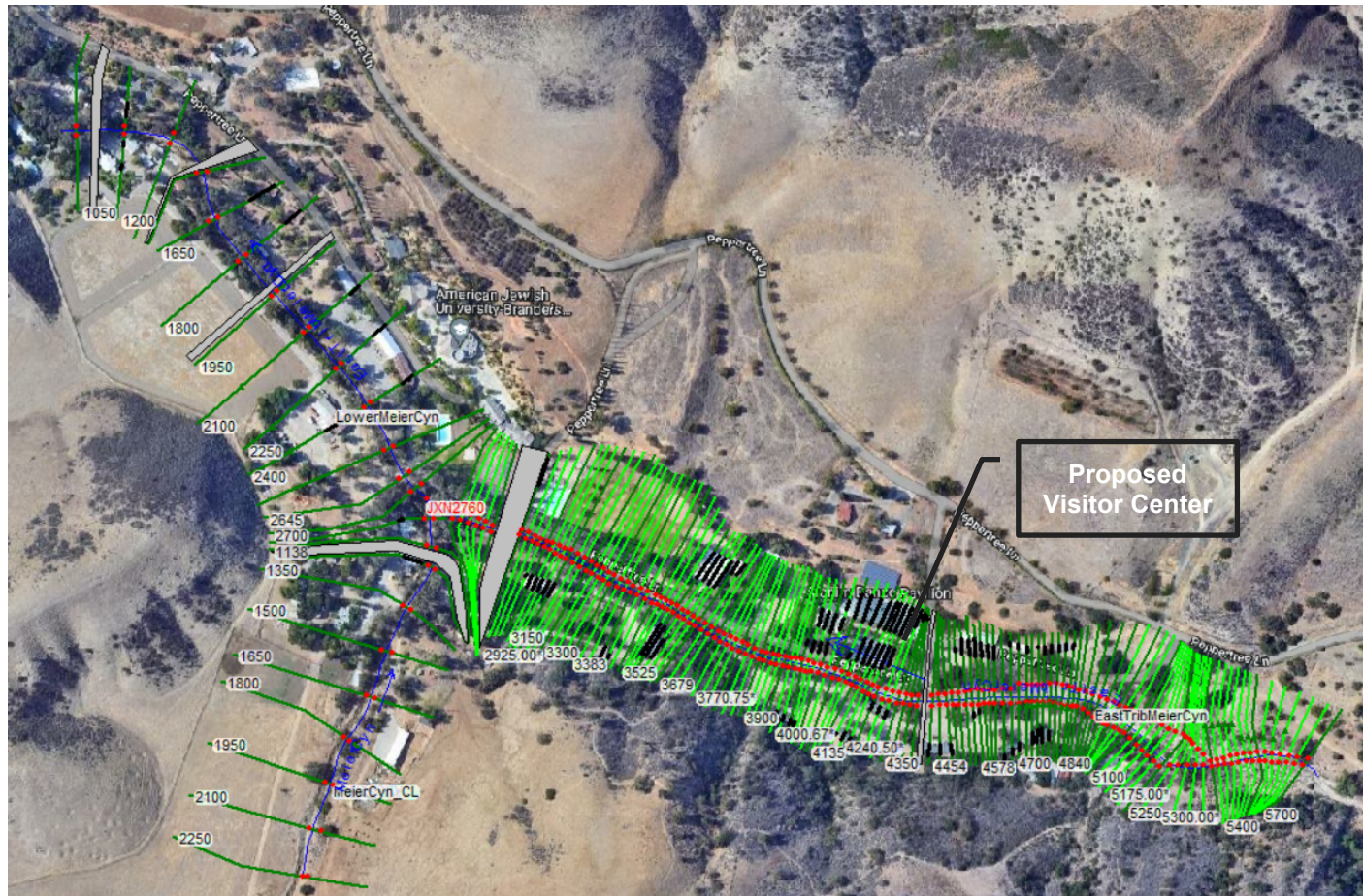
Figure 3. Schematic of 1D HEC-RAS hydraulic model geometry for Meier Canyon Creek Study Reach, proposed condition
