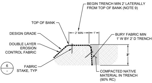
5 TOP TRENCH DETAIL SECTION VIEW SCALE: 1" = 2'
