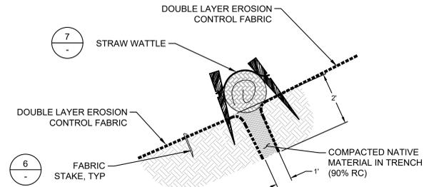
4 MID-SLOPE TRENCH DETAIL SECTION VIEW SCALE: 1" = 2'
