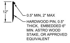
6 FABRIC STAKE DETAIL SECTION VIEW SCALE: 1" = 1'
