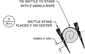
7A WATTLE DETAIL SECTION VIEW SCALE: 1" = 2'
