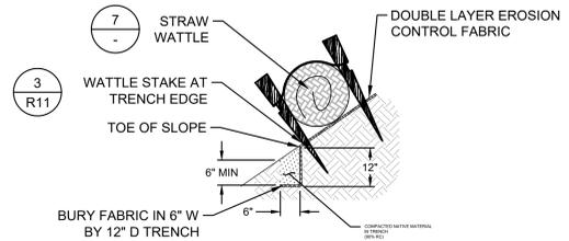
3 BOTTOM TRENCH DETAIL SECTION VIEW SCALE: 1" = 2'
